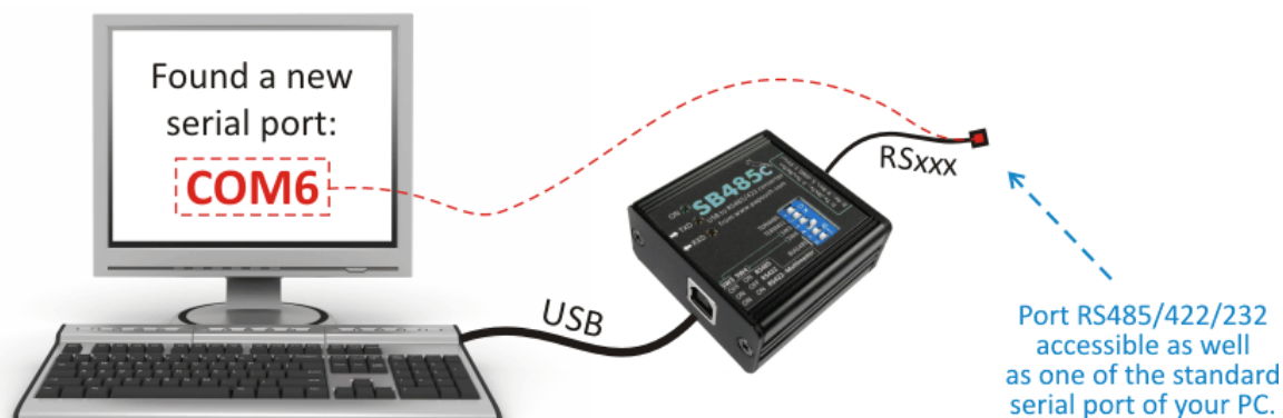
Fig. 1 – After connecting, “a virtual serial port” is created in your PC. Within the system it acts like a standard serial COM port.
