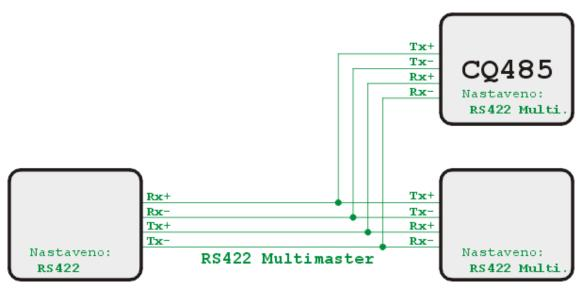
Fig. 11 - Example of a system with RS422 line interconnection in the multimaster mode.
