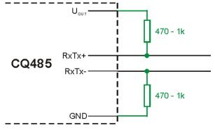
fig. 6 - external resistors
