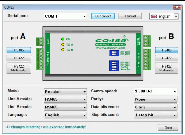
Fig. 4 - Configuration software
