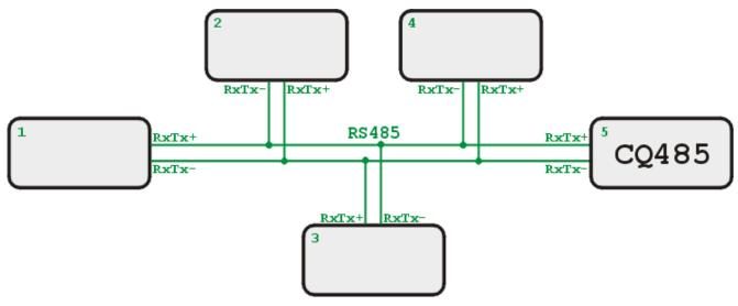
Fig. 9 – An example of a system with an RS485 line interconnection.
