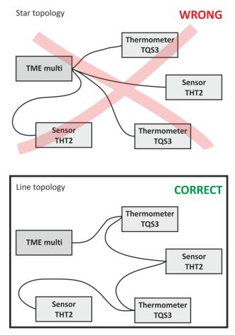
Fig. 4 – correct connection of the system
